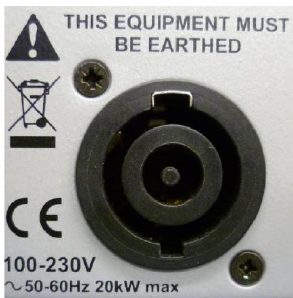
Mains inlet markings
