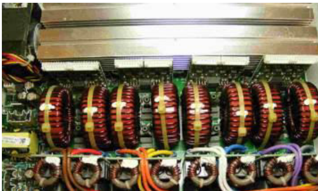
8 channel amplifier PCB
