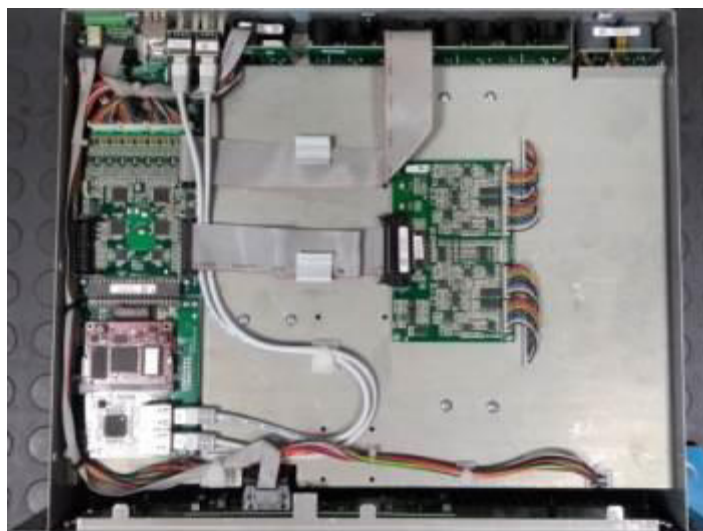
4 channel with Dante card fitted
