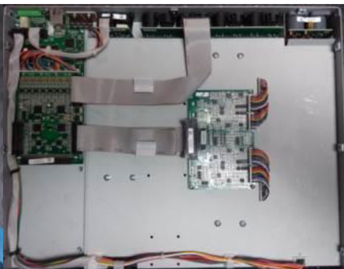
4 channel without Dante card fitted
